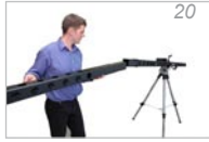
Fig. 20. Connection of extension segment (2) with main segment (3)
