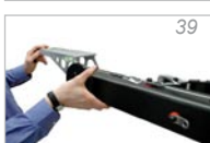
Fig. 40. - 42. Installing the right outrigger-rope (the one without the turnbuckle) for lateral bracing
