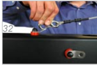
Fig. 34. Retightening the tower-rope with rope clamping fixture
