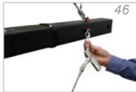
Fig. 47. Hanging up the outrigger-rope into the outrigger
