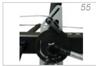
Fig. 55. Angle change with pulley
