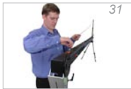
Fig. 31. - 33. Hooking the tower-rope at the head segment (•)
