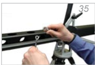
Fig. 35. - 36. Installing the steering rope for the version 8. „L“
