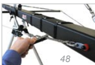
Fig. 48. Closing the turnbuckle of the outrigger-ropes
