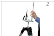
Fig. 2 - 4 Assembly of the crane support
