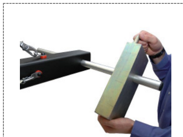
53. Gewichte aufladen. "Kran in die Waage bringen" / Load up the counterweights for taring the crane, secure weights on tubes with securing clips
