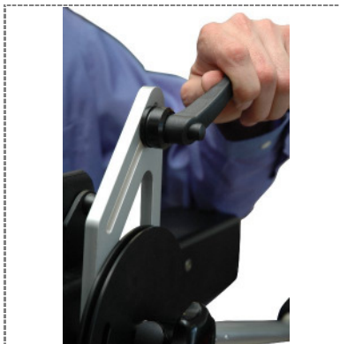
17. Umlenkhebel befestigen / Fix lever securely.
